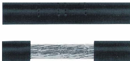
穿刺效果图 Photo of thrusting result
